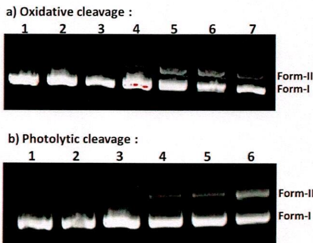
Fig. 8. Gel electrophoresis images of oxidative (a) and photolytic cleavages (b) of supercoiled pBR322 DNA (0.2 mg, 33.3 mM) in 5 mM Tris-HCl/NaCl buffer (pH = 7.2) by all compounds. In oxidative cleavage , Lane 1, DNA control: Lane 2, DNA + \text{H}_2\text{O}_2 (1 mM): Lane 3, DNA + \text{H}_2\text{O}_2 (1 mM) + \text{H}_2\text{L} (20 mM): Lane 4, DNA + \text{H}_2\text{O}_2 (1 mM) + Co(II) complex (20 mM): Lane 5, DNA + \text{H}_2\text{O}_2 (1 mM) + Ni(II) complex (20 mM): Lane 6, DNA + \text{H}_2\text{O}_2 (1 mM) + Cu(II) complex (20 mM): Lane 7, DNA + \text{H}_2\text{O}_2 (1 mM) + Zn(II) complex (20 mM). In photolytic cleavage , Lane 1, DNA control: Lane 2, DNA + \text{H}_2\text{L} (20 mM): Lane 3, DNA + Co(II) complex (20 mM): Lane 4, DNA + Ni(II) complex (20 mM): Lane 5, DNA + Cu(II) complex (20 mM): Lane 6, DNA + Zn(II) complex (20 mM).
